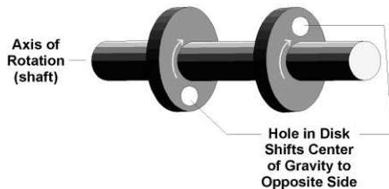
The goal in a 2-plane dynamic balance is for both discs to have the same static balance. Again, looking from the end of the shaft at the system below, we can see that the system is statically balanced; and looking at the location of the balancing stock removal of both disks we can see that it is also dynamically balanced in 2-planes.
