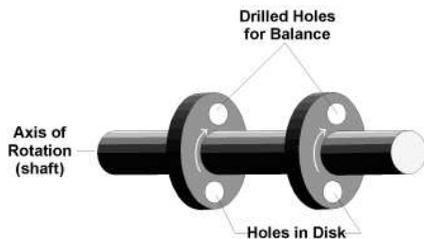
Of course, most dynamic balancing is more complex than this simplified example, since it isn't very likely that the two discs will have the same amount of imbalance. The magic is in getting both the location and amount of stock removal right so that the center-of-gravity of both discs is the same.
